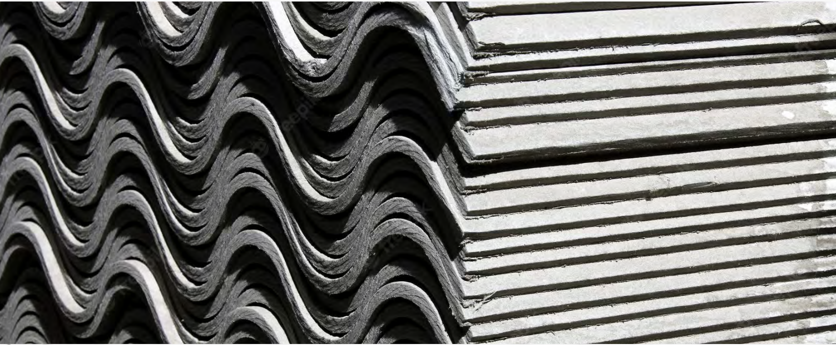
Asbestos microfibrils, which can be found in asbestos cement structures, are classified as a toxic material.
